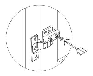
2) If doors fails to close flush, turn screw on rear of hinge to loosen. Adjust doors and retighten screw.
