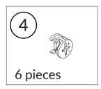
With arrow facing downward, insert cam locks (#4) into bottom of parts B & C then turn to lock.
