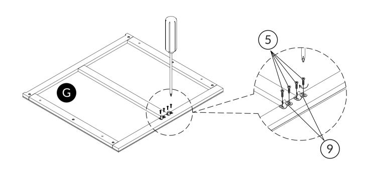
Attach roller catch stike (#9) to part G with screws (#5). Raised lip should face inward.
